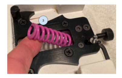
e) Place the spring pin (12) from the top of the bridge into the other end of the spring (3) while still supporting the spring with your finger.
